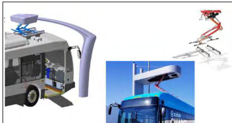
Figure 8. Infrastructure-mounted Cross Rail Connection (Source: Kosowski 2018)
