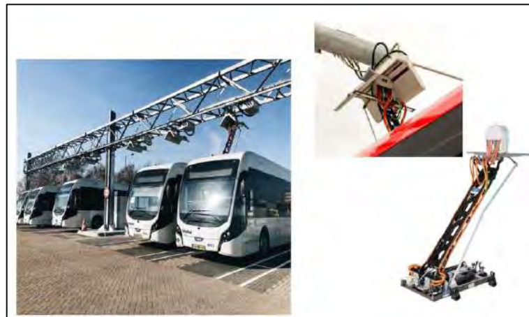
Figure 10. Vehicle-mounted Pantograph Connection (Source: Kosowski 2018)
