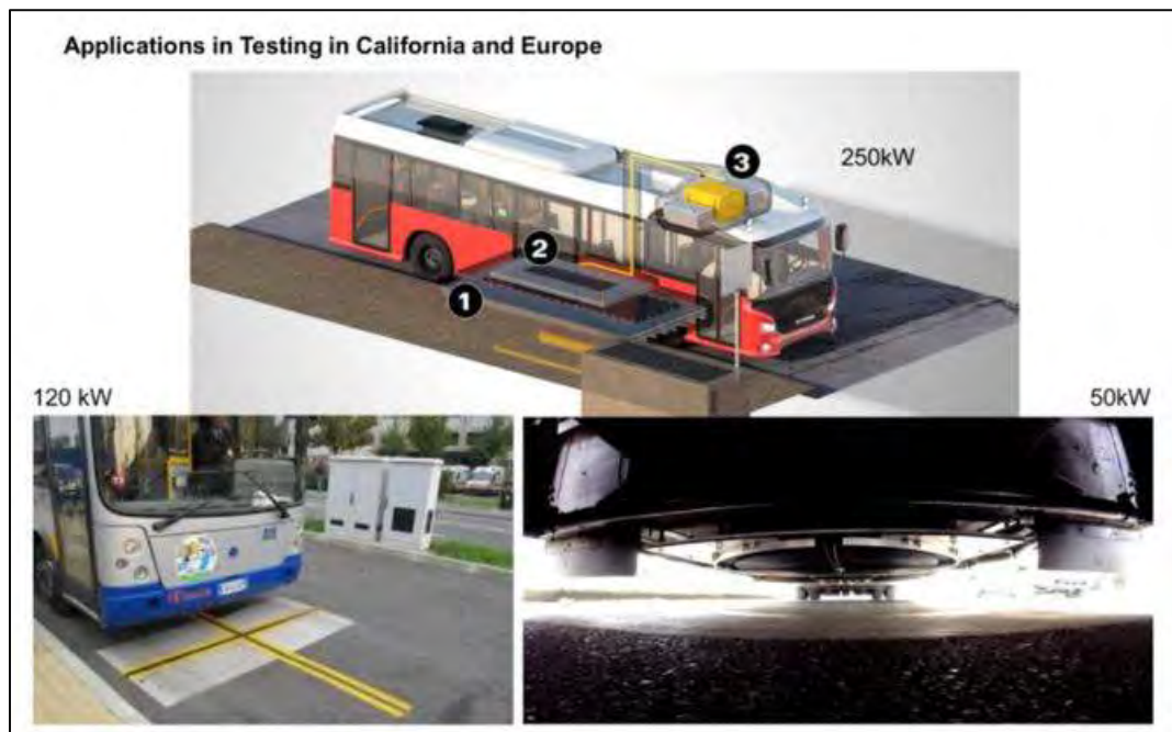
Figure 12. Wireless Power Transfer Pilot Projects (Source: Published in Green Car Congress, originally ConduTix Wämpfler, Scania, and WAVE Technologies)
