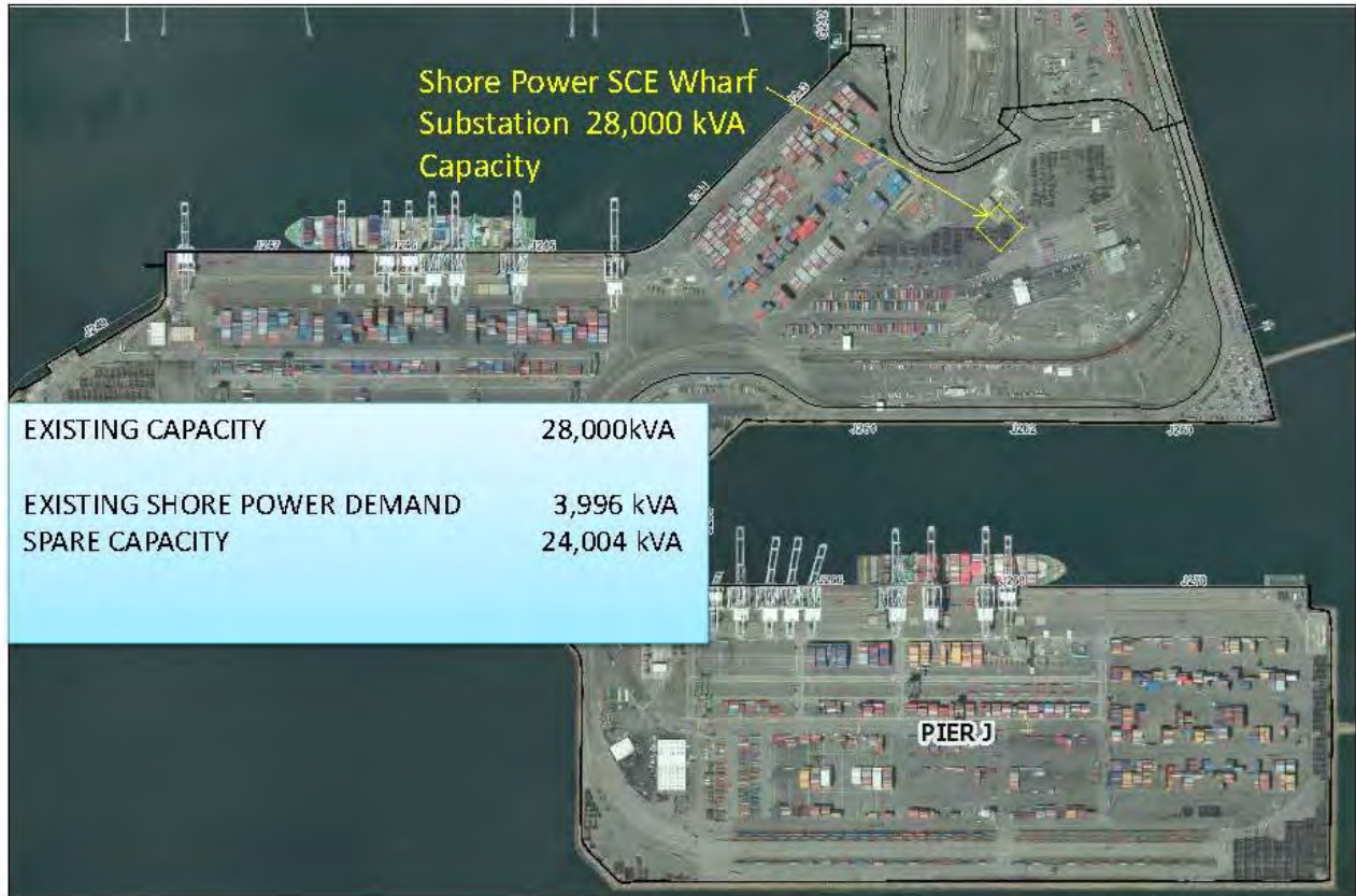
Figure 5: Pier J PCT – Electrical Capacity and Demand
