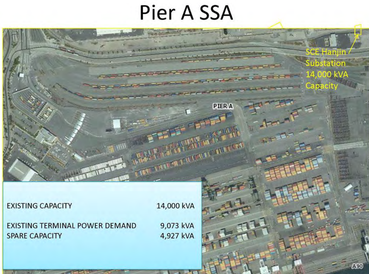
Figure 1: Pier A SSA– Electrical Capacity and Demand
