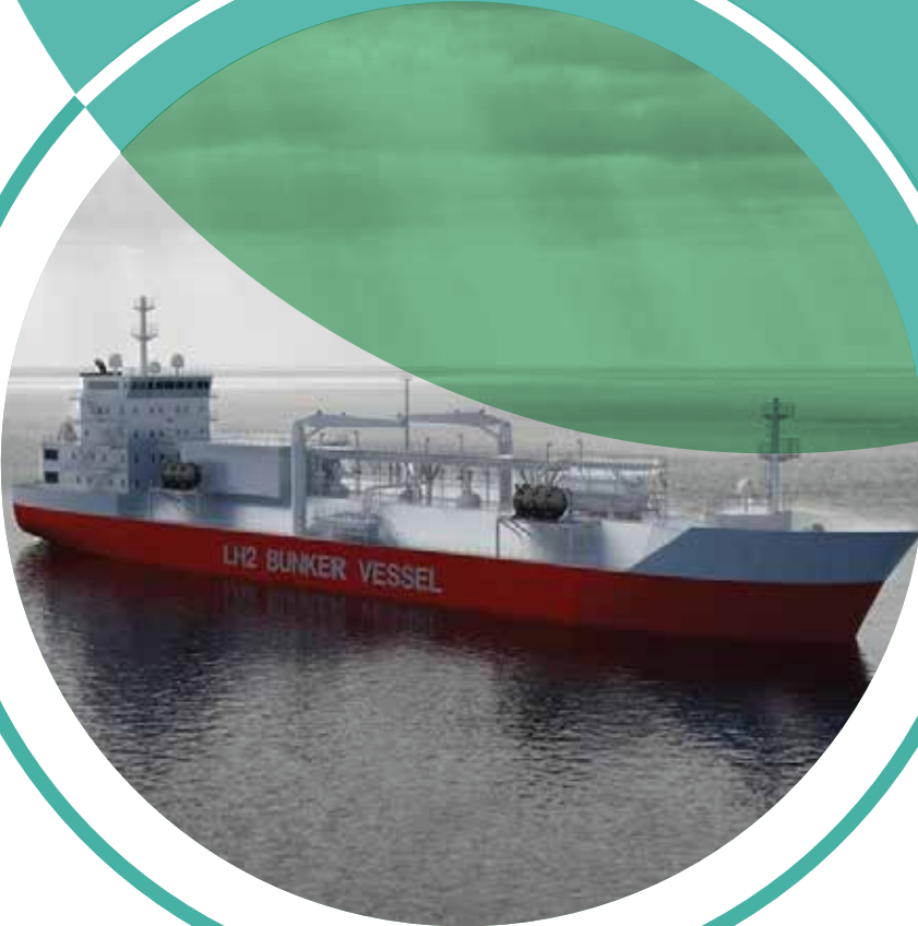
Moss Maritime's rendering of liquefied hydrogen bunker vessel developed by Moss Maritime, Wilhelmsen Ship Management, Equinor, and DNV-GL. Photo: Moss Maritime
