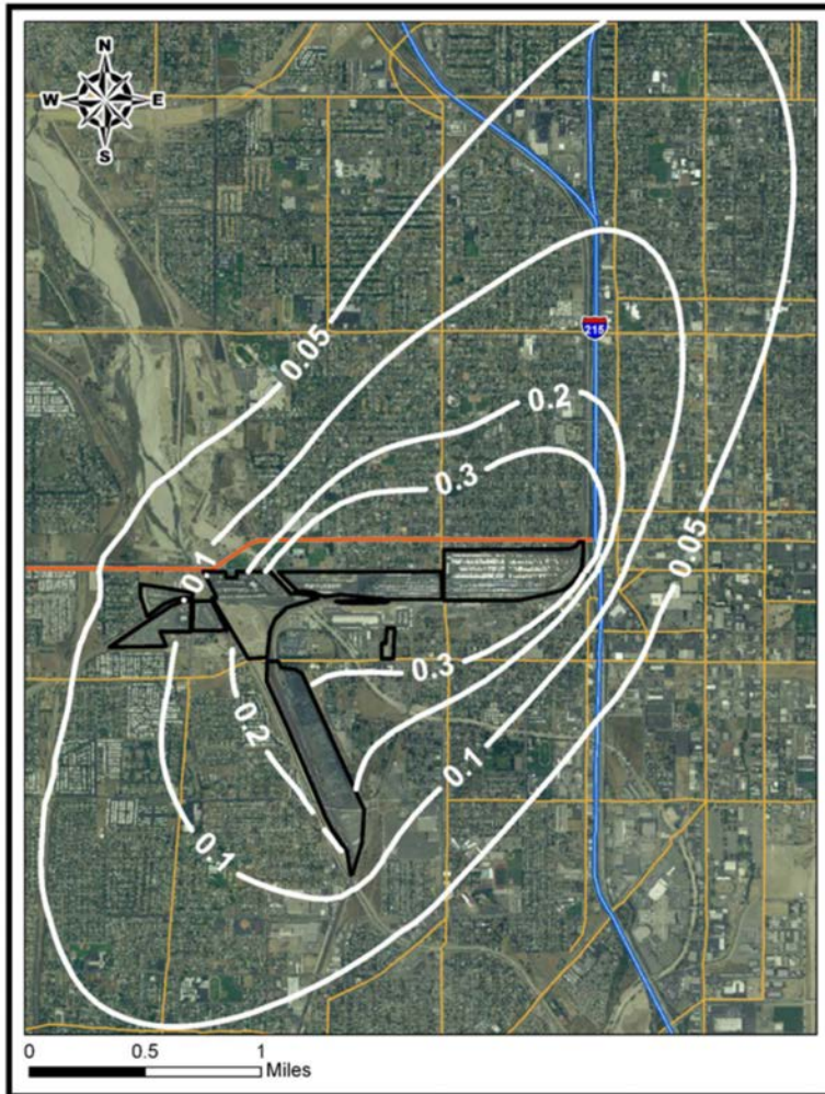
Figure 9: Estimated non-cancer health risks (Hazard Index) associated with operations at the BNSF San Bernardino Railyard.
