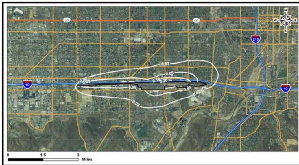
Figure 17: Estimated non-cancer risk (Hazard Index) associated with diesel emissions at the UP Colton Railyard, according to the 2008 CARB HRA (REF63).
